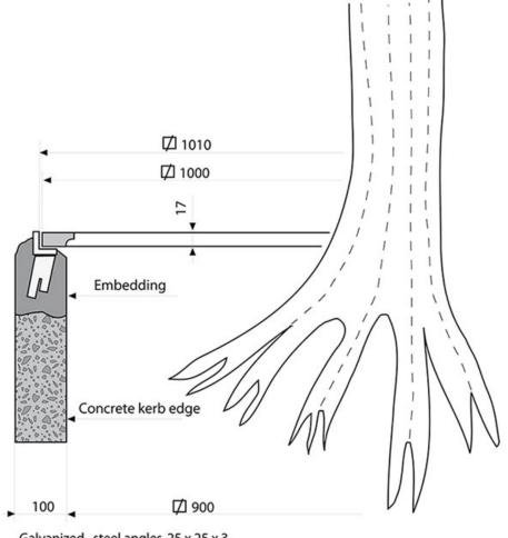
Galvanized steel angles  $25 \times 25 \times 3$  Inclined legs with  $15^{\circ}$  length 55mm
